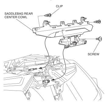
34. Remove the parts as shown.
