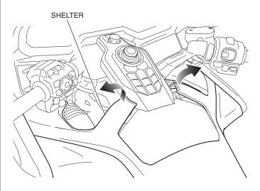
12. Insert the helmet holder into the gap as shown. <Right side>
