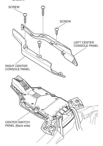
18. Remove the center console garnish as shown.
