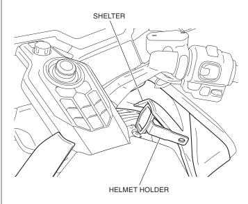
13. Remove the screw and clip as shown.
